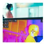
If a high temperature is detected, SMS, email and/or single/multi-camera smart alerts are sent to individuals and care teams via monitors, mobile devices or the Internet. With a detection time of less than one second and accuracy of  $\leq \pm 0.5$ °F, it's now possible to identify individuals with a fever before they enter your facility so you can keep your workplace open while protecting both employees and visitors.
